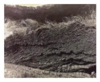
This image shows the outer part of the bag filter. It still has white areas. The outer bag is a support layer for the internal melt blown filter cartridge and is not expected to be full of contaminate, which happens with low efficiency filter bags
