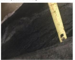
This image is a close up of the same media showing a complete loading of the filter cartridge
