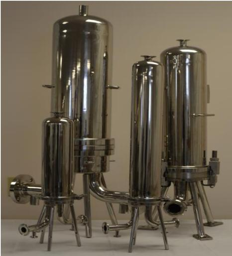
Single and multi-round housings are constructed of 316L stainless steel designed with standards for filtration applications requiring high purity production. Design characteristics minimize hold up volumes, provide for easy draining and cleanability. External surfaces mechanically polished and internal surface is acid washed for a consistent, easy care finish. Available to accommodate multiple configurations and up to 36 individual cartridges.
