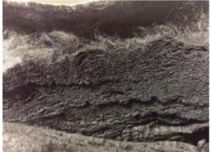
This image shows the outer part of the bag filter. It still has white areas. The outer bag is a support layer for the internal melt blown filter cartridge and is not expected to be full of contaminate, which happens with low efficiency filter bags
