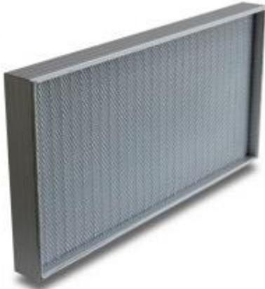
HT pleat filters are designed as a pre filter operating at high temperatures up to 500°F/260° C, with low pressure drop and long service life. Filters are classified with MERV8/G4/EU4 efficiency. They are made with a pleat distribution of 13 pleats per linear foot and are recommended to operate up to 2000 CFM. These filters are available in 45mm (2") and 95mm (4") depths. Filter face area can be custom made in many dimensions and the maximum recommended pressure drop is 1.2" w.g./300 Pa.
