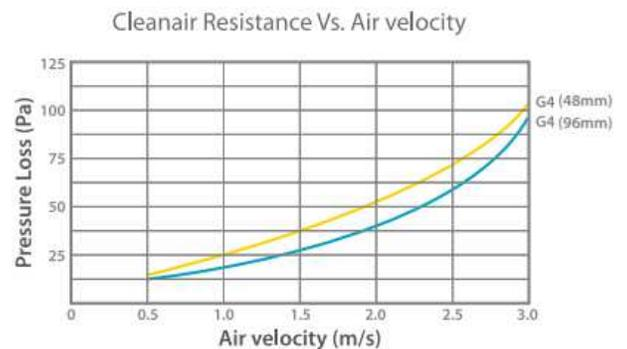
**Pro-Clean POLY-PLEAT** filters are cleanable / washable panel filters made up of non woven, high lofted synthetic (polyester) filter media and are available in various efficiency grades ranging from G2 to F5. POLY PLEAT filters offer very high dust holding capacity combined with lower resistance than the other types of similar grade panel filters.
