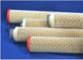
Elements offer economical, high quality Beta rated filtration for applications where “absolute” filters are required. Elements are available in cellulose, glass-cellulose and microglass media with a variety of end configurations and sizes. The pleated design ensures high contaminant retention due to the large surface area. Elements are available in ratings from 2 to 30 microns.
