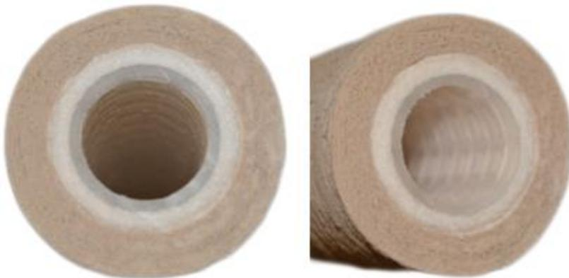
The 4-zone technology allows the larger particles to be trapped in the outer most layers. The inner most layer is where the true efficiency rating is achieved. The two images show how there is a consistent dirt loading pattern throughout the life of the filter.
