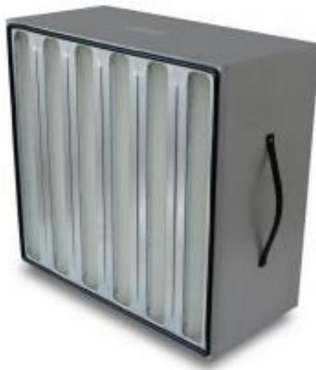
4V operates at very high air velocity up to 2000 CFM if required delivering a very low pressure drop. The V shaped arrangement allows more air flow per filter wherein a standard filter replacement can save up to 30% energy savings. Filters are light weight and its fully plastic body makes it incinerable as well.
