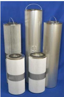
Designed for filtration of water, water based fluids, and a wide range of chemicals. These filter cartridges stand up to continuous use in water based fluids without the softening and/or deterioration common with many resin impregnated paper cartridges. These elements are made with an advanced synthetic polyester media, which allows high flow rates with low pressure drops as well as excellent temperature resistance.
