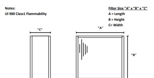
\*\*Glass media HEPA filters can flow either direction. The direction of airflow noted on filter is the direction the filter was tested before leaving the factory.
